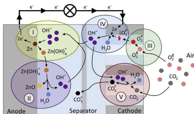
Schematic of alkaline ZAB operation from *J. Power Sources*, 360 (2017) 136-149.
