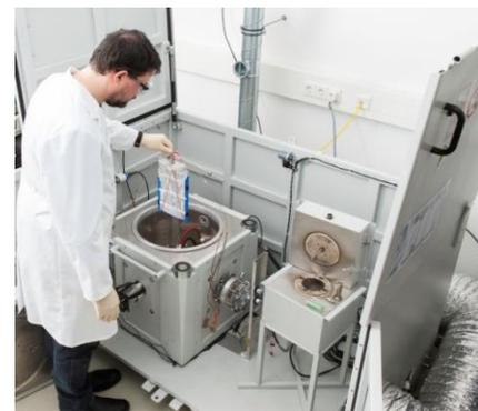
Figure 4. Two accelerating rate calorimeters (ARC) for safety testing of cells and packs.
