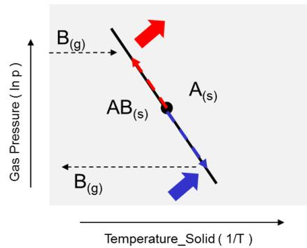
Figure 3. Reversible gas-solid reactions allow the temperature to be a function of the gas pressure.
