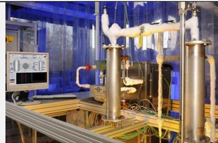
Figure 5. Test stand for thermal upgrade of waste heat at  $T > 140\text{ }^{\circ}\text{C}$  (DLR).
