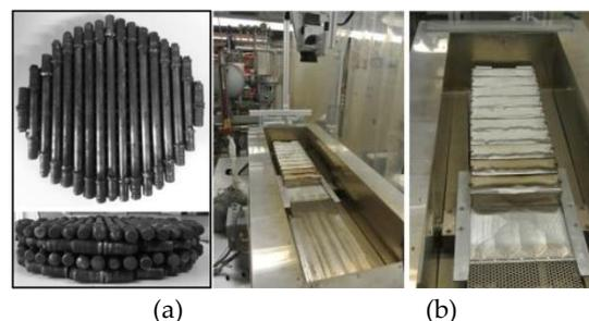
Figure 2. HT-LHTES (a) encapsulated PCM [2] and (b) lab-scale testing device [2].
