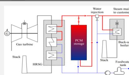
Figure 4. LTES integration in a Co-gen plant [4].
