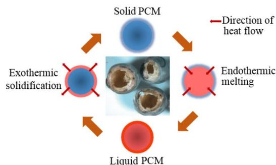
Figure 2. PCM working concept (LHTES) with 5 mm high-temperature PCM capsule with voids shown in the centre [1].
