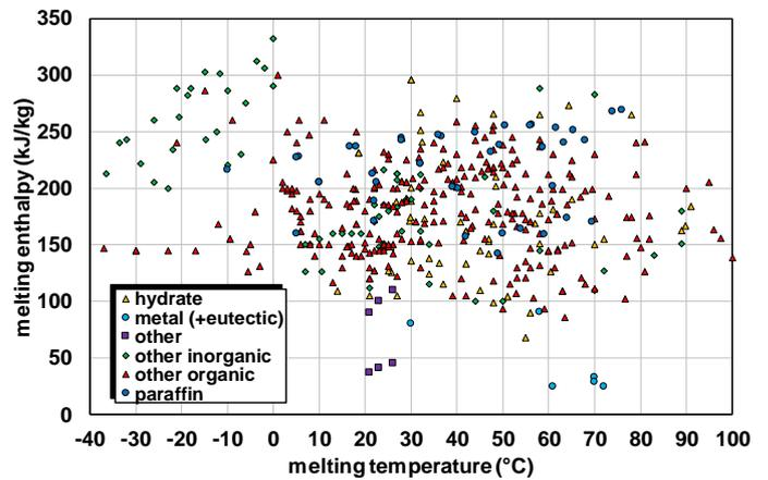
Fig. 1: Latent heat vs. phase change temperature of various low temperature PCMs (data [1-5]).
