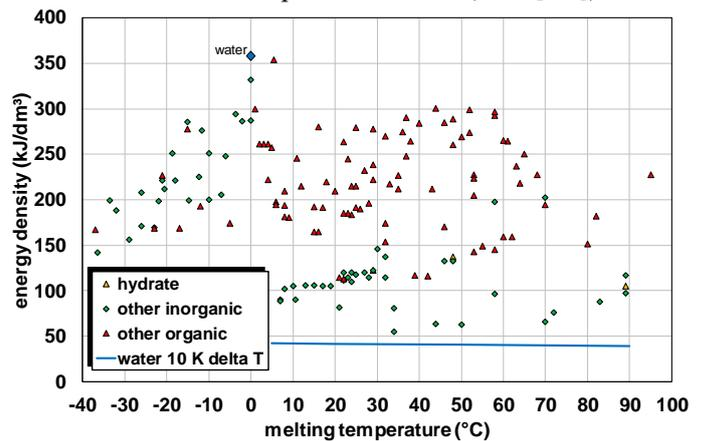
Fig. 2: Energy density vs. phase change temperature of various PCMs (data [1-5]).
