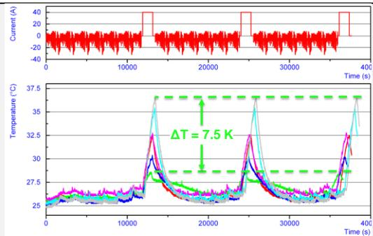
Figure 3: Peak shaving with low temperature PCMs during quick charging of batteries (source: AIT)
