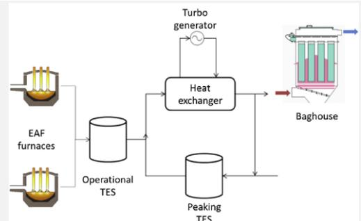
Fig.4. Steel electric arc furnace energy recovery and storage system [4].
