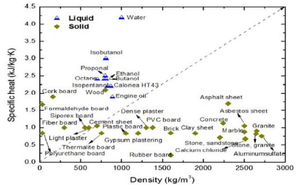
Fig. 1. Thermal properties of sensible heat materials [1].
