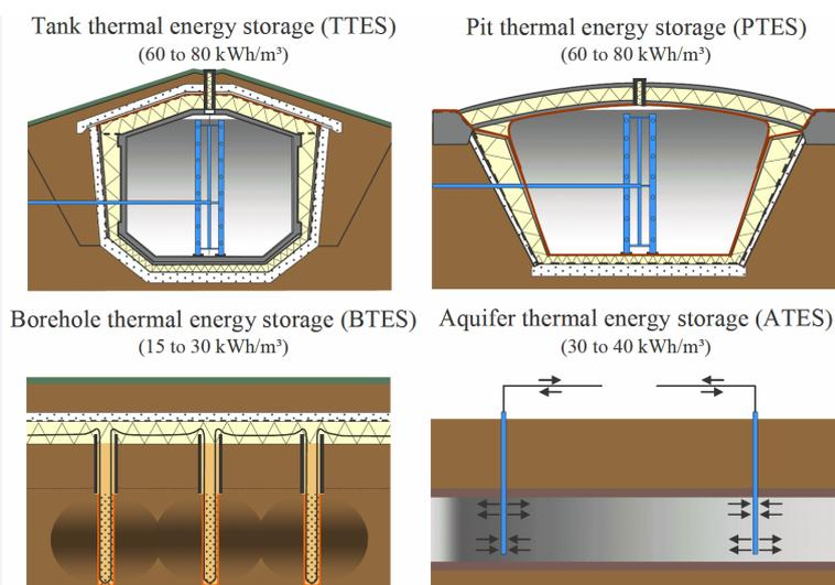
Figure 1. Methods of sensible heat thermal energy storage [1]
