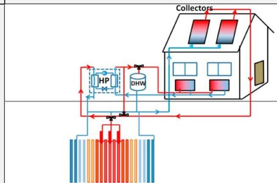
Figure 6. Borehole thermal energy storage [6].
