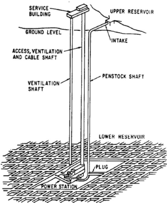
Figure 2. Grid gallery underground pumped lower reservoir example [3]
