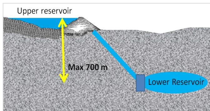
Figure 1. Underground pumped hydro scheme [8]
