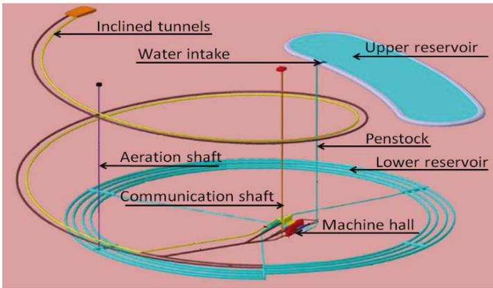
Figure 4. Scheme of a 1000 MW pumping plant with a spiral shape gallery underground reservoir [7]
