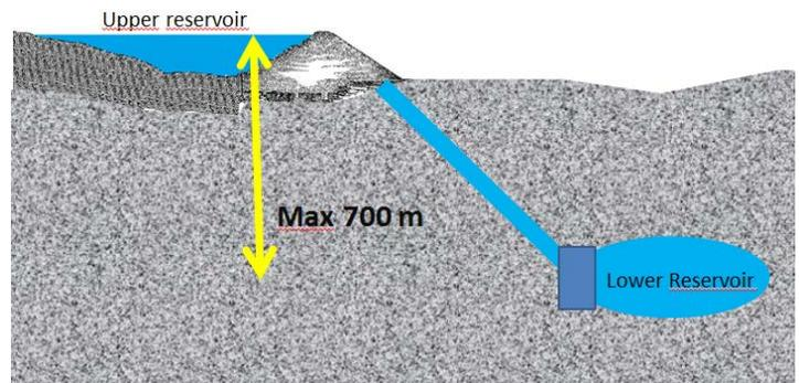
Figure 1. Underground pumped hydro scheme [11]
